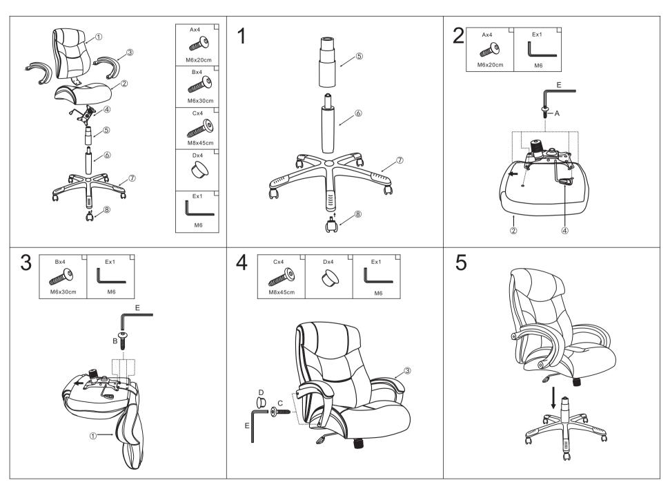
Notice:Please tighten screws up initially using fingers only to avoid cross threading the screws
